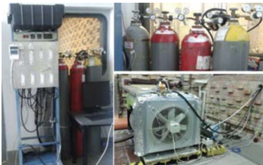
Fig. 1. Test station with engine and supply system
