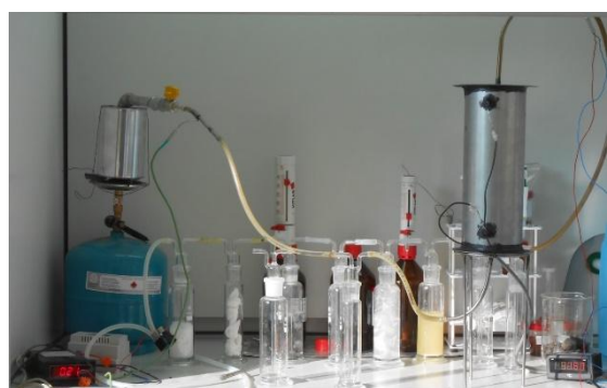
Figure 1. Gasification and gas conditioning system, used in experiment no. 2
